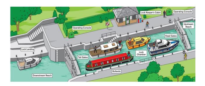
Not all of the locks on the river are the same. Some have wooden beams that have to be pushed open by hand. The others like this picture, are opened mechanically
